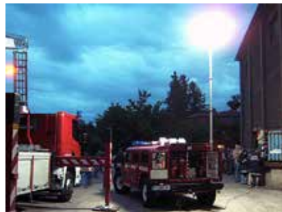
Fire brigade truck with on board lighting balloon
